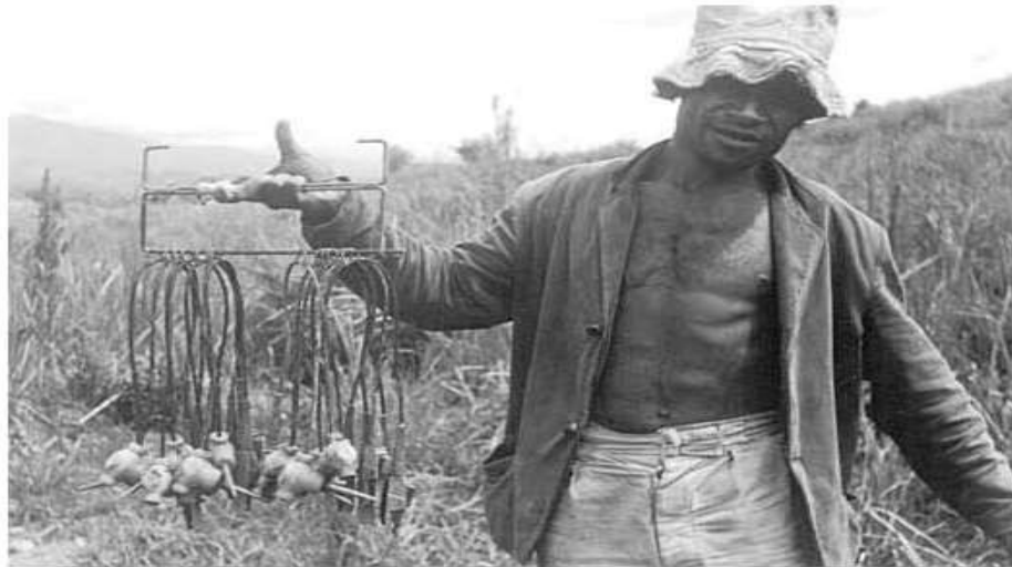
Fig. 3.3: Geophone Carrying Frame in Use, Papua New Guinea
