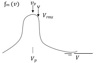
The figure shows the schematic Maxwellian velocity distribution fm(v) of an ideal electron gas. The velocity with the highest probability,  $V_P$  is lower than the mean velocity v and the root mean square velocity,  $V_{rms}$
