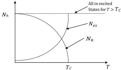
The figure above shows the plot of  $N_{ex}$  and  $N_{g}$  as a function of temperature according to Einstein model.
