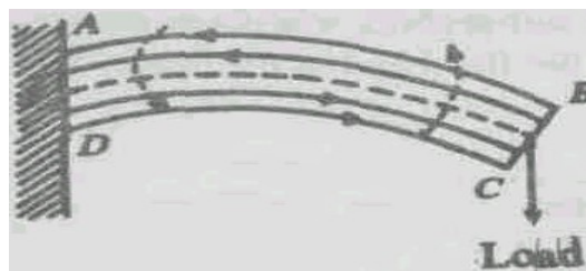
Fig. 6.5: When the beam is bent then in the upper half, the restoring forces opposing extensions in the filaments act inwards towards the fixed end. While, in the lower half, the restoring forces opposing contractions act outwards. The moments of these two sets of forces about the neutral axis are directed in the anticlockwise (indicated by dotted arrows) direction and thus oppose the bending of the beam.
