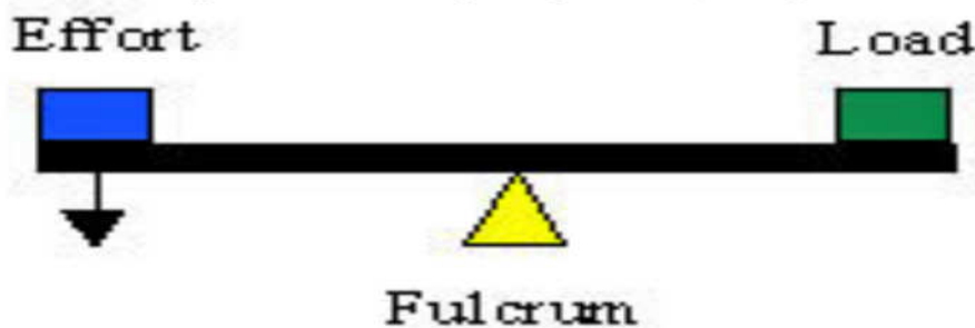
Figure 26: A Simple Lever showing effort, fulcrum and load.
