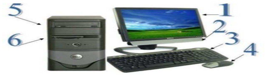
1) Monitor. 2) Speaker. 3) Keyboard. 4) Mouse. 5) CPU (Central Processing Unit 6) - Floppy Drive
