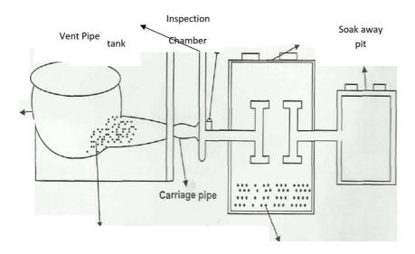
This is one of the most popular and acceptable methods of excreta disposal. It requires water to function effectively since all liquid waste and faecal matter are removed by gravity assisted by this flow of water. It consists of the following major parts:
