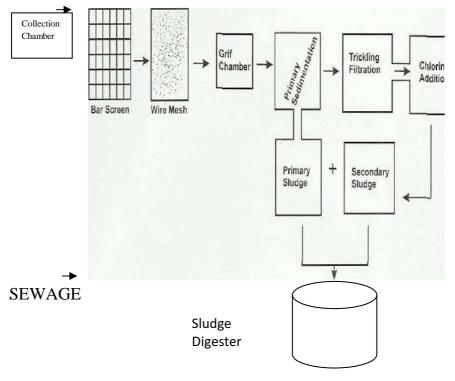
There are so many levels and process in sewage treatment. These processes comprise of biological treatment and chemical treatment which ever type must operate under primary and secondary level treatment.
