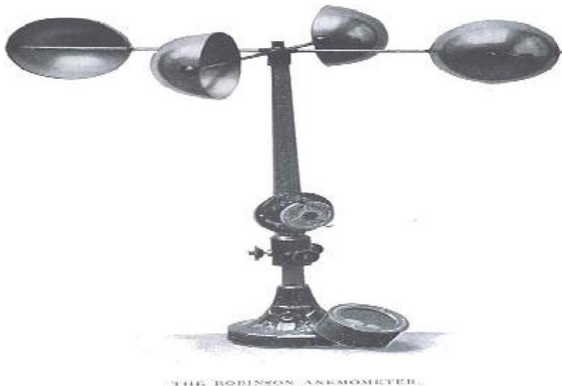
Fig. 1.6: A Typical Four Cup Anemometer
