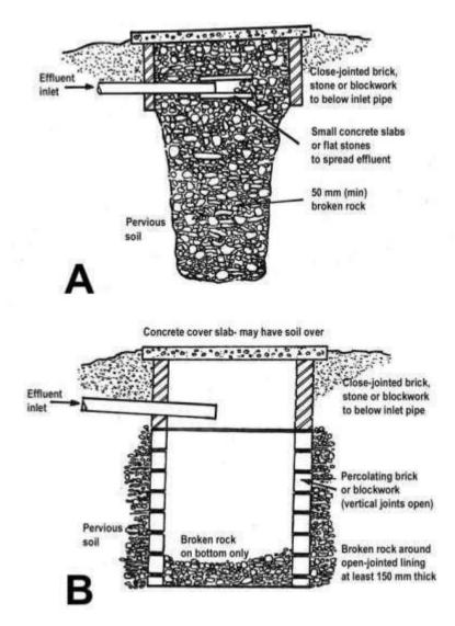
**Fig. 6:** Unlined (A) and lined (B) Soakage pits with effluent inlets Source: Assar (1971) in WHO (2002)
