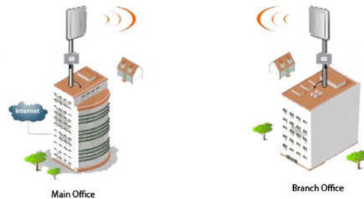
Fig. 3.1: Point-to-point wireless system
