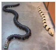
*Figure 8:* Two robot snakes. Left **one** has 64 motors (with 2 degrees of freedom per segment), the right one 10.
