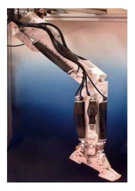
*Figure 5:* A robotic leg powered by Air Muscles
