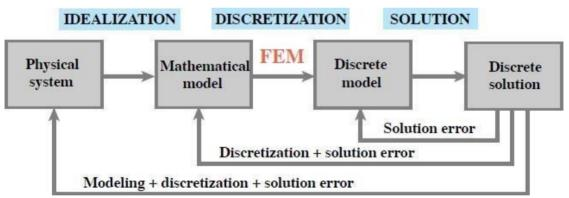
Figure 1: Steps of the physical simulation process: idealization, discretization and solution.
