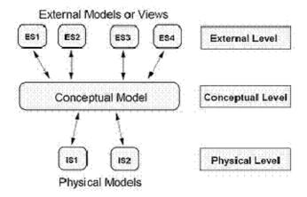
Fig. 6: ANSI/SPARC three level architecture.
