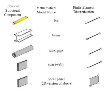
Figure 4. Examples of primitive structural elements
