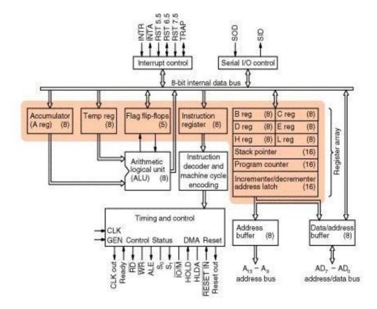
Figure 1: Architecture of 8085 Microprocessor
