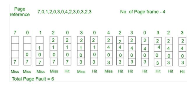
Initially all slots are empty, so when 7 0 1 2 are allocated to the empty slots —> 4 Page faults 0 is already there so —> 0 Page fault.
