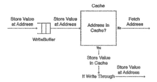
Figure 4.13: Operation of a memory cache write
