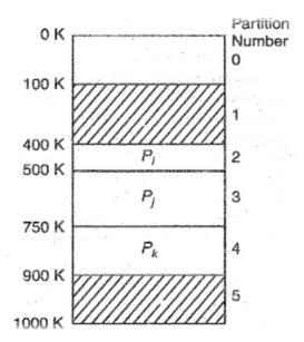
Applying first fit method, the process P will be allocated in partition 1 which will result 300 - 70 = 230 gap of unusable memory until process P terminates or swapped out of the memory. Applying best fit algorithm, process P will be allocated in partition 5 which will result 100 KB - 70 KB = 30 KB of unusable memory units.
