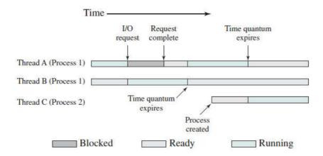
Figure 2.7: Multithreading on a uniprocessor
