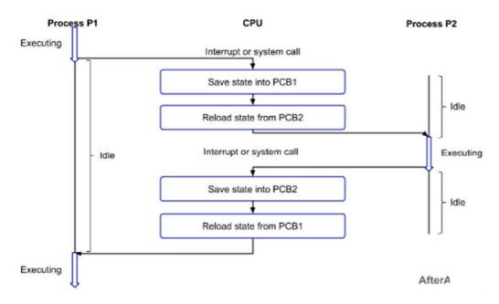
Figure 2.1b: Switching between two processes
