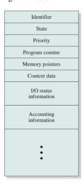
Figure 1.2: Process Control Block diagram
