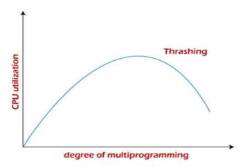
Figure 4.17: CPU utilization against degree of multiprogramming
