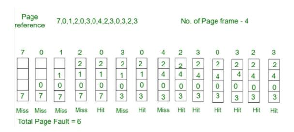
Initially all slots are empty, so when 7 0 1 2 are allocated to the empty slots —> 4 Page faults 0 is already their so —> 0 Page fault.
