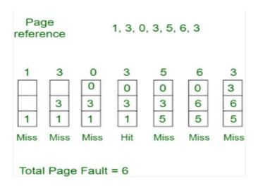
Initially all slots are empty, so when 1, 3, 0 came they are allocated to the empty slots —> 3 Page Faults.
