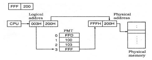
If the capacity of physical memory is m and the size of each page is p then the number of frames in the physical memory will be
