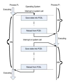
Figure 2.1: CPU Switching from one process to another
