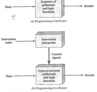
Figure 3.1 Hardware and Software Approaches
