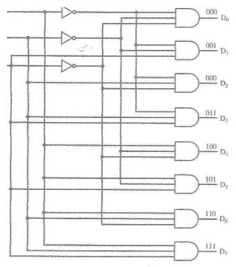
are 20.15 Decoder with 3 Inputs and  $2^3 = 8$  Outputs
