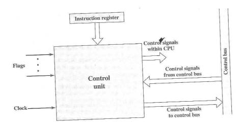
Figure 3.2.1 is a general model of the control unit, showing all of its inputs and outputs. The inputs are
