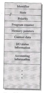
Figure 8.8 Process Control Block
