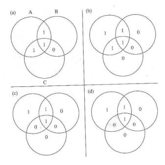
The simplest of the error-correcting codes is the *Hamming code* devised b: Richard Hamming at Bell Laboratories. Figure 5.8 uses Venn diagrams to illustrate the use of this code on 4-bit words (M=4). With three intersecting circles, there as even compartments. We assign the 4 data bits to the inner compartments (Figure
