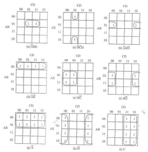
Figure 20.9x, based on Table 20.3, illustrates the simplification process. If any isolated 1s remain after the groupings, then each of these is circled as a group of 1s. Finally, before going from the map to a simplified Boolean expression, any group of 1s that is completely overlapped by other groups can be eliminated. This is shown in Figure 20.9b. In this case, the horizontal group is redundant and may be ignored in creating the Boolean expression.
