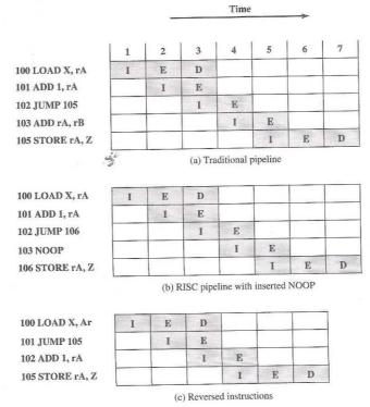
Figure 13.7 Use of the Delayed Branch
