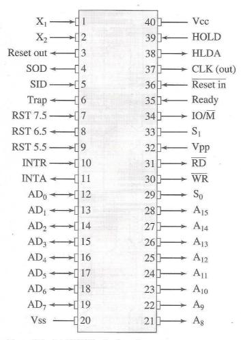
Figure 15.8 Intel 8085 Pin Configuration
