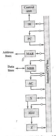
Figure 15.6 CPU with Internal Bus
