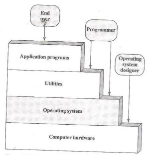
Figure 8.1 Layers and Views of a Computer System
