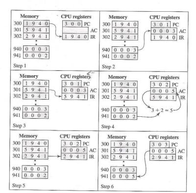
For example, the PDP-11 processor includes an instruction, expressed physically as ADD B,A, that stores the sum of the contents of memory locations B into memory location A. A single instruction cycle with the following steps
