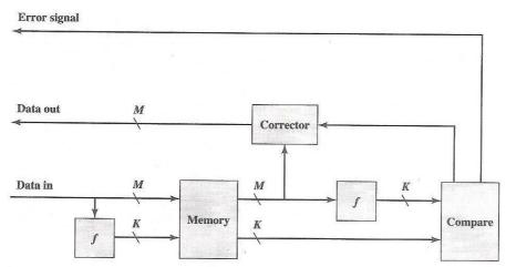
Figure 5.7 Error-Correcting Code Function
