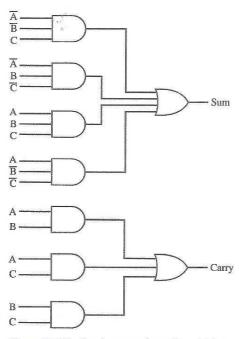
Figure 20.20 Implementation of an Adder
