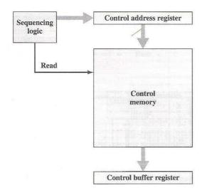
from the control unit. Thus, *reading* a microinstruction from the control memory is the same as *executing* that microinstruction. The third element shown in the figure is a sequencing unit that loads the control address register and issues a read command.
