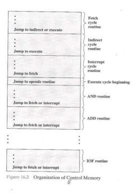
The control memory of Figure 16.2 is a concise description of the complete operation of the control unit. It defines the sequence of micro-operations to be performed during each cycle (fetch, indirect, execute, interrupt), and it specifies the sequencing of these cycles. If nothing else, this notation would be a useful device for documenting the functioning of a control unit for a particular computer. But it is more than that. It is also a way of implementing the control unit.
