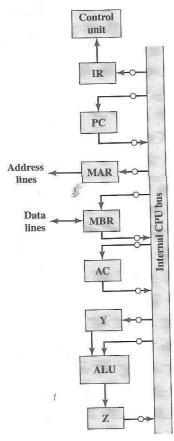
Gates and control signals are provided for movement of data onto and off the bus from each register. Additional control signals control data transfer to and from the system (external) bus and the operation of the ALU.
