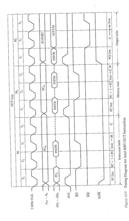
addressed memory module places the contents of the addressed memory vocation on the address/data bus. The control unit sets the Read Control (RD) signal to indicate a read, but it waits until  $T_3$  to copy the data from the bus. This gives the memory module time to put the data on the bus and for the signal levels to stabilize. The final state,  $T_4$ , is a bus *idle* state during which the processor decodes the instruction. The remaining machine cycles proceed in a similar fashion.
