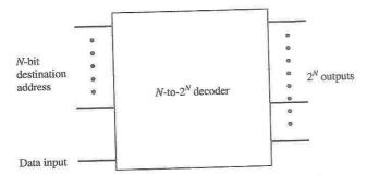
Figure 20.17 Implementation of a Demultiplexer Using a Decorder
