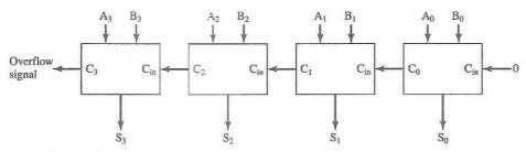
Figure 20.19 4-Bit Adder
