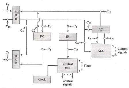
Figure 15.5 Data Paths and Control Signals
