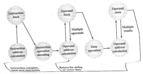
Figure 3.6 Instruction Cycle State Diagram
