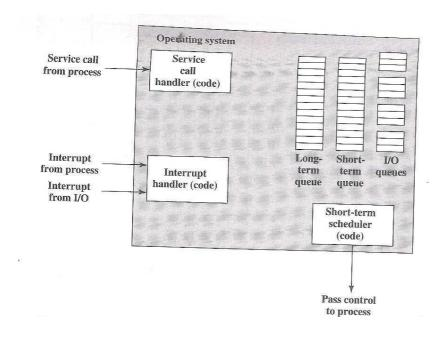
and scheduling of processes. The OS receives control of the processor at the interrupt handler if an interrupt occurs and at the service-call handler if a service call occurs. Once the interrupt or service call is handled, the short-term scheduler is invoked to select a process for execution.
