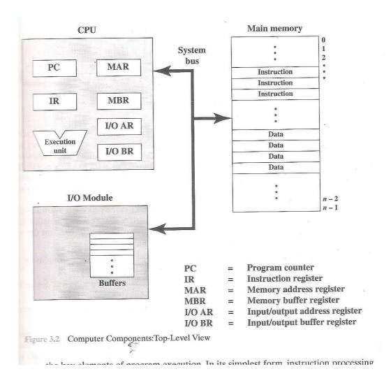
the key elements of program execution. In its simplest form, instruction processing consists of two steps: The processor reads (*fetches*) instructions from memory one at a time and executes each instruction. Program execution consists of repeating the process of instruction fetch and instruction execution. The instruction execution may involve several operations and depends on the nature of the instruction (see, for example, the lower portion of Figure 2.4).
