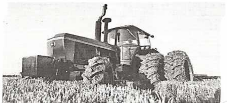
FIG. 16-7. Two-wheel drive tractor with optional front wheel power drive. (Courtesy Deere and Company)
