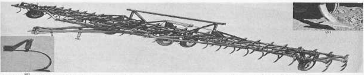
Fig. 18-27. Pull-type field cultivators have become very popular secondary tillage tools for field finishing or seedbed preparation working 2 to 5 in [50 to 125 mm] deep. Outside wings fold for transport and flex for even penetration across the full width of the unit. (a) Shanks are spring-cushioned (insert) for vibrating action and trash removal. Shank points are 1\frac{1}{2} \times \frac{1}{2} \times 11 in [44.45 \times 6.35 \times 279.4 mm] and are used for shattering crust ahead of planting. (b) V-sweeps are 4 to 12 in [101.6 to 304.8 mm] wide and are used for weed control, leaving crop residue on or near the surface. (Deere & Co.)
