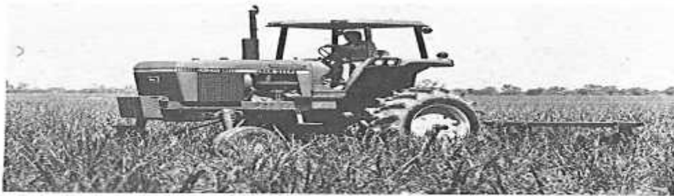
2. Tractor with extra-high clearance for sugar cane. (Courtesy Deere and Company)
